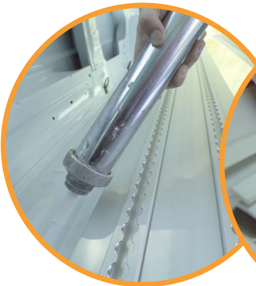
A non-toxic, single-component adhesive applied directly onto the degreased vehicle bottom provides easy and flexible installation of the floor profiles which, again, saves you some time. Part no. 70278 Even the degreaser is non-toxic. Simple alcohol will do just fine.
